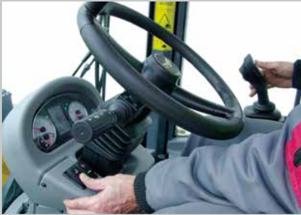
Electrical proportional adjustment of the hydraulic performance of the 3rd and 4th circuits.
